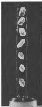
Above (Fig. 4): Perfect synthetic quartz crystal. Original seed plate visible inside. Right (Fig. 5): Series of growing quartz crystals in harness used in bomb. Below (Fig. 6): Spurious seeds resulting from a leak in the crystal-growth bomb.
