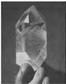
Above (Fig. 4): Perfect synthetic quartz crystal. Original seed plate visible inside. Right (Fig. 5): Series of growing quartz crystals in harness used in bomb. Below (Fig. 6): Spurious seeds resulting from a leak in the crystal-growth bomb.
