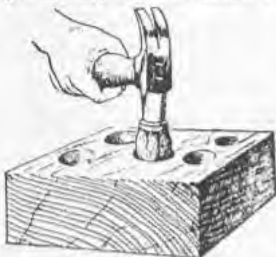
Holes in Block for Nuts
