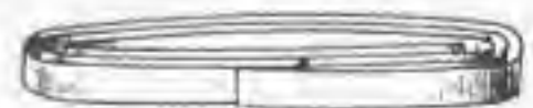
The Filled Edge on the Coiled Metal Retains the Sand Particles as It is Rubbed over the Glass Surface
