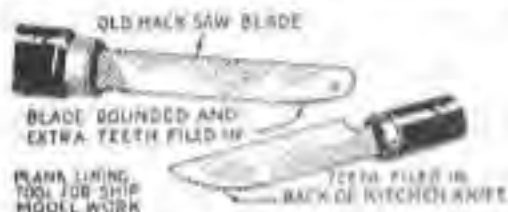
FIG. 20.—Either an old hack saw blade or a common paring knife can be converted into a tool for making slight grooves to represent planking on ship model hulls.
