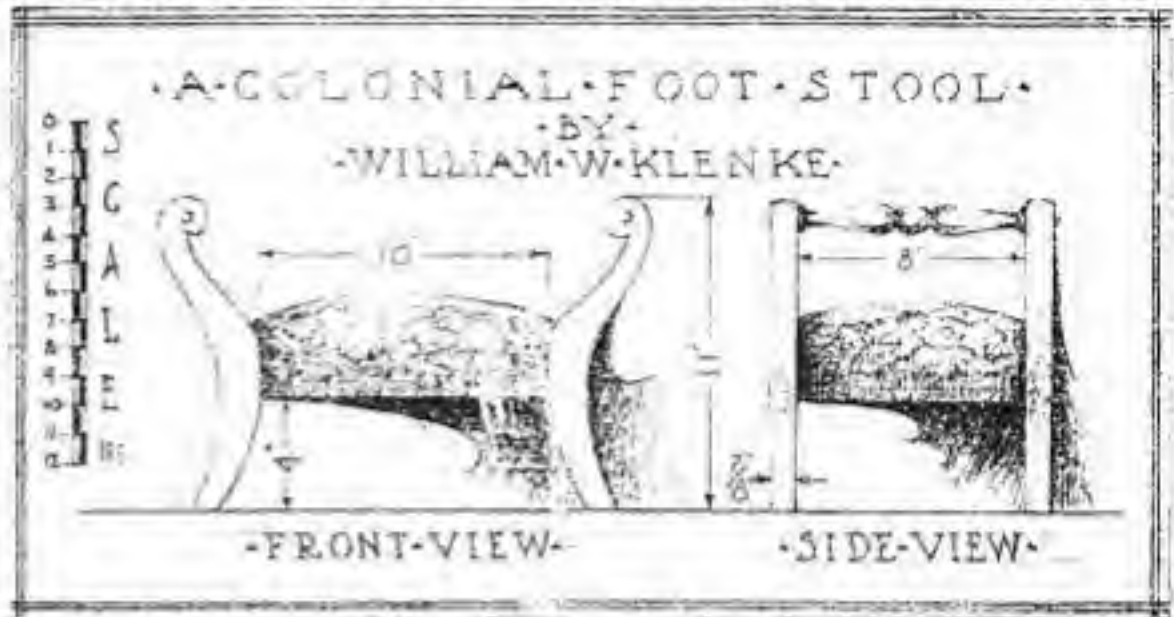
FIG. 2.—Original pencil sketch of the footstool, which was made as a preliminary to illustrating the various steps in machining for parts. For details, see the drawings in Fig. 3.
