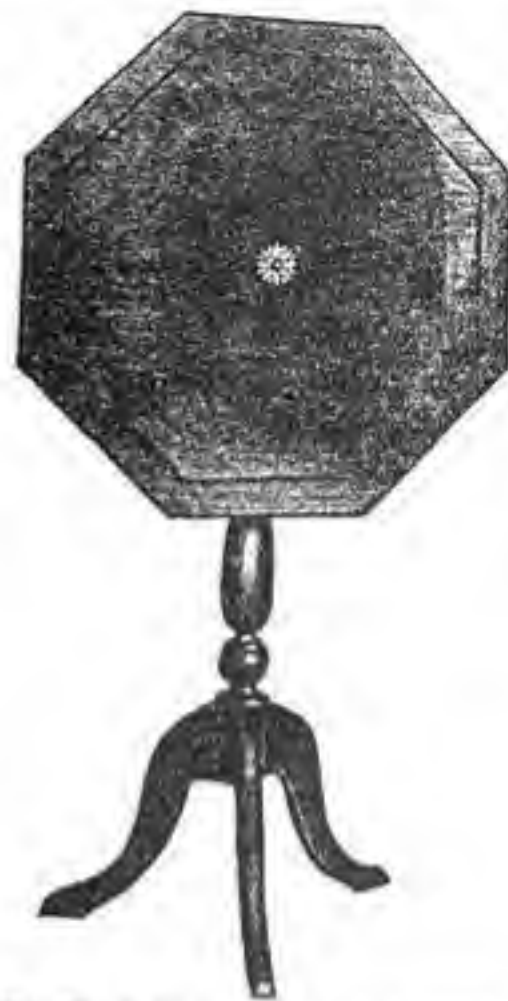
FIG. 29.—A turned-top table with a turned column. The top is decorated with an inlay insert and border.
