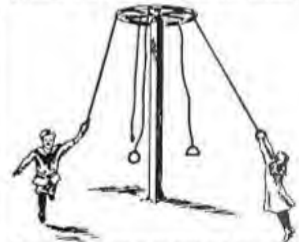
The Ropes being Tied to the Wheel Rim will Easily Turn around the Pole
