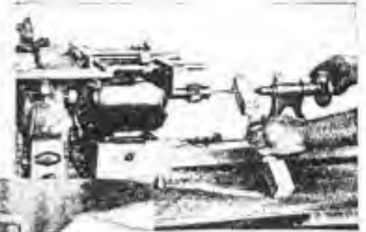
FIG. 15 (above).—Boring the dowel holes. Should holes have to be bored all the way through the stock, a block is bored and fitted over the tailstock spindle to save the bit from damage.
