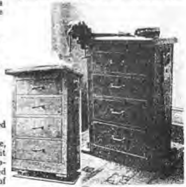
FIG. 9.—The apartment-size cabinet workbench ready for use (above) and raised on casters (at left). It can be rolled away and stored in a closet.
