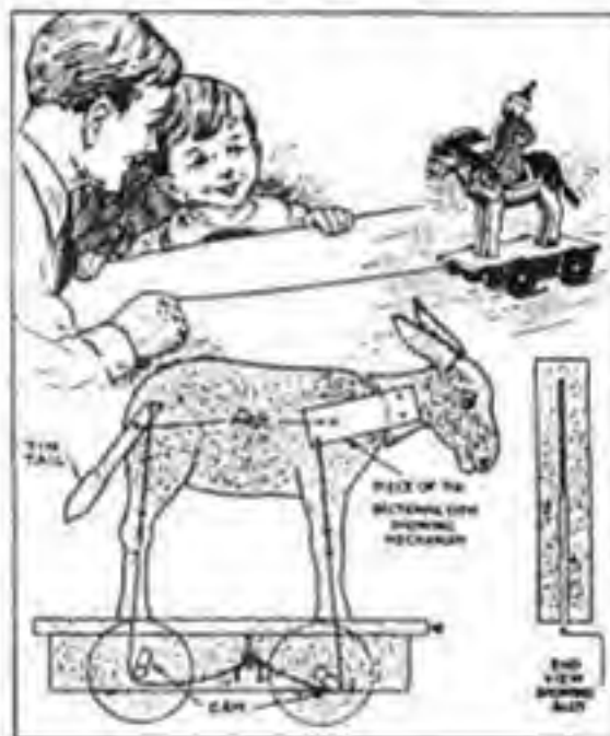
A Toy Donkey That Wags Its Tail and Nods Its Head, When Drawn across a Table, Has a Simple Mechanism That Makes It Easy to Construct
