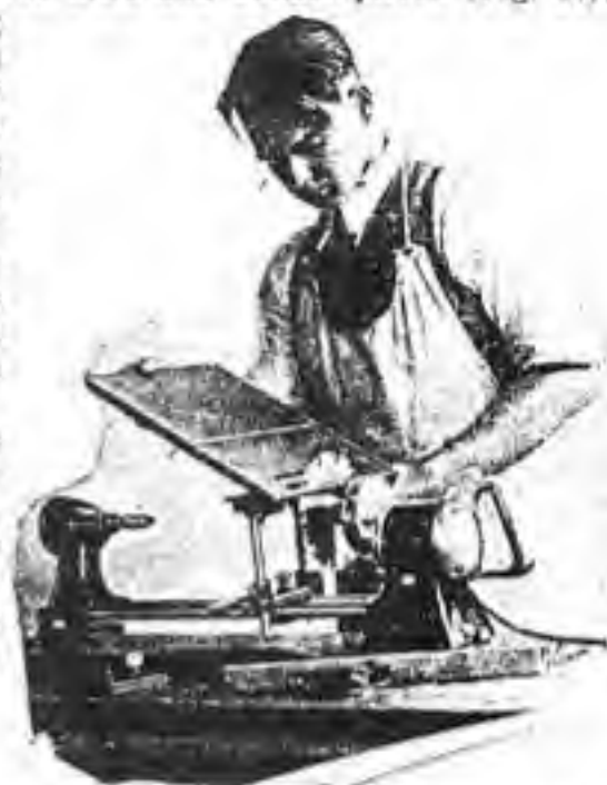
FIG. 24.—Cutting miters by tilting the table at 45 degrees and placing the molding on its edge.
