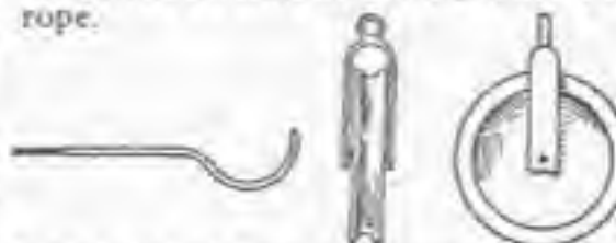
The Yoke of the Pulley is so Arranged as to Make It Move in All Positions on the Hook
