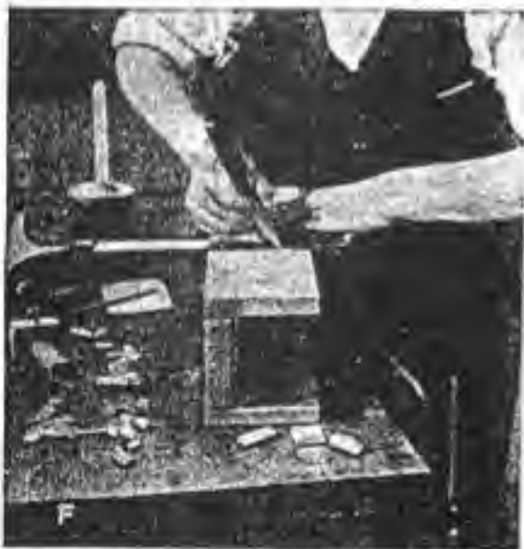
FIG. 35.—Steps in making a miter box of wood. The work must be done with extreme care, and the cuts should be made with the saw which is to be used with the box.
