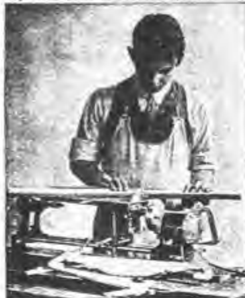
FIG. 23.—The common method of curving miters with the cut-off fence at 45 degrees and the table level.
