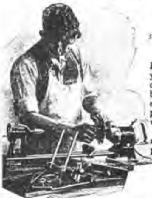
FIG. 22.—The new blade is mounted so that the top teeth point toward the operator.
