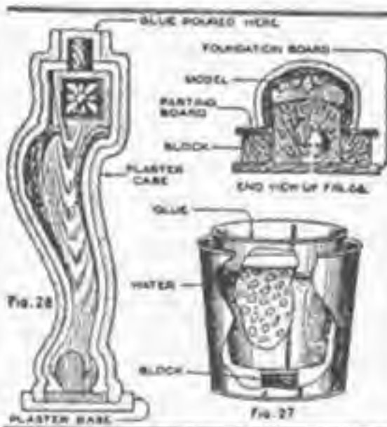
Mold in Position, Ready for Filling with Glue: Figure 27 Shows How the Glue should be Melted for Large Pieces
