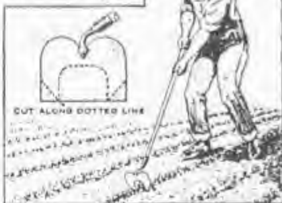
A Fork-Shaped Hoe. Made from the Standard Garden Hoe. Makes It Possible to Save Time by Working on Both Sides of a Row of Seedlings at the Same Time
