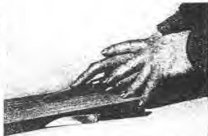
FIG. 21.—Two special tools made as shown in Fig. 20 for cutting fine grooves to represent the planks of other divisions in ship models and similar work.
