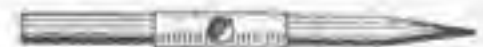
A Torch Made of Glass and Rubber Tubing, to be Used on an Ordinary Gas Jet
