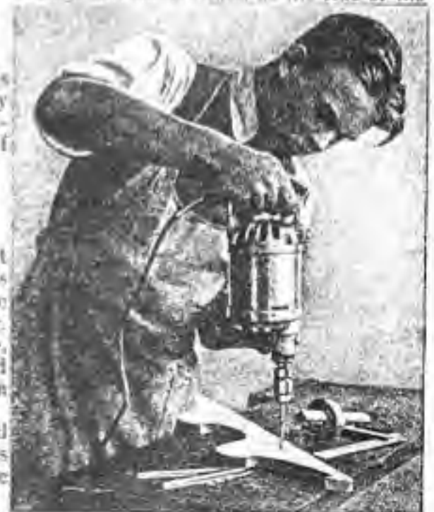
FIG. 33.—Some types of portable electric saw motors can be easily dismantled and used as electric hand drills for drilling screw holes, making holes for inserting a jet saw, and other light work.
