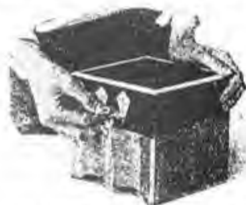
FIG. 7.—Gummed tape is used to make guide for sandblasting certain parts of the design before painting.
