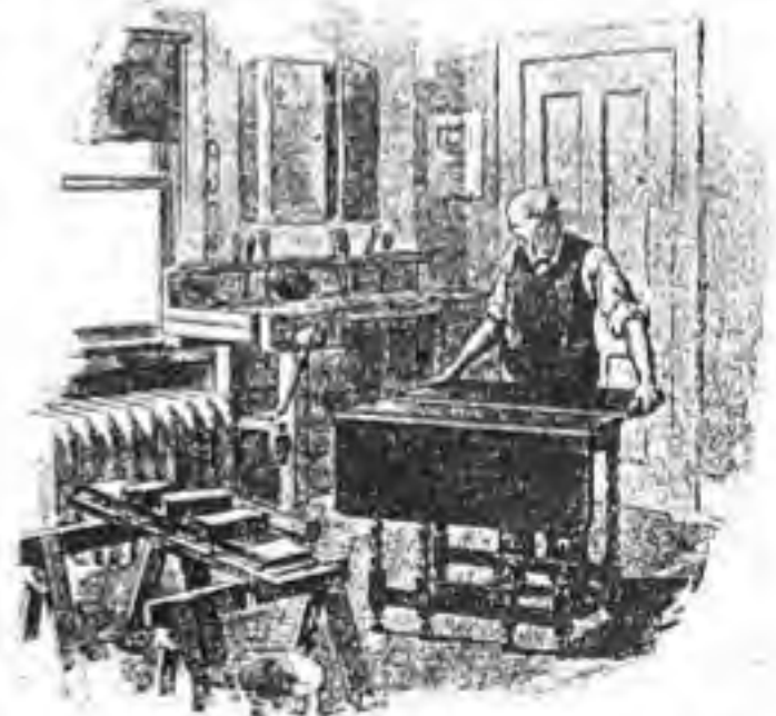
FIG. 8.—Repairing antique furniture is one of the most interesting and profitable of trades. Even badly warped boards can be re-straightened in time by the application of moisture and pressure as shown at the left.
