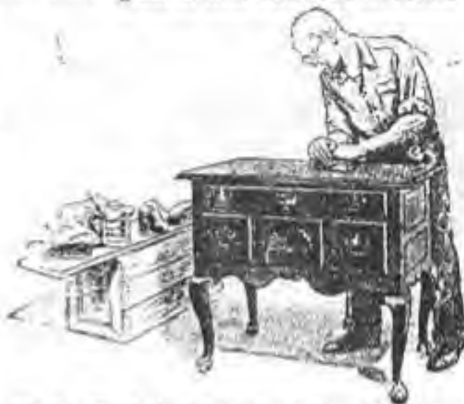
FIG. 24.—The final polish is given to the oiled and waxed top of a low box with a rubbing block.
