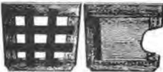
FIG. 16.—Whether webbing or a thin board is used to make a foundation for upholstery on a flat seat frame, it is applied on the underside.
