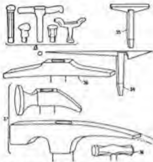
FIG. 15.—A set of stakes, and raising and planishing hammers. A shoemaker's hammer will serve for planishing, and a brick hammer makes an excellent hammer for raising operations.
