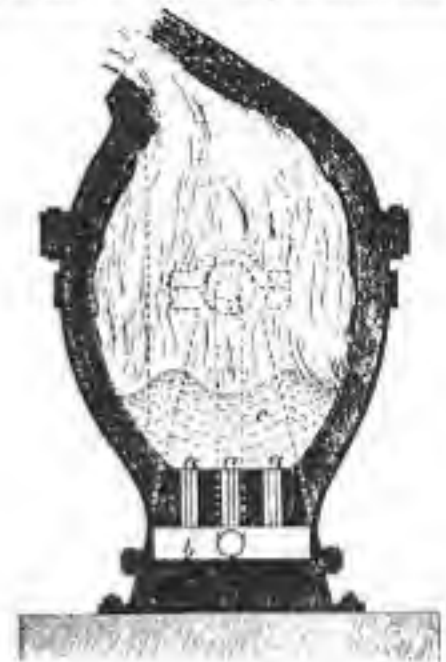
Bessemer Converting Vessel : a, a, a, tuyeres; b, air-space; c, molten metal.
