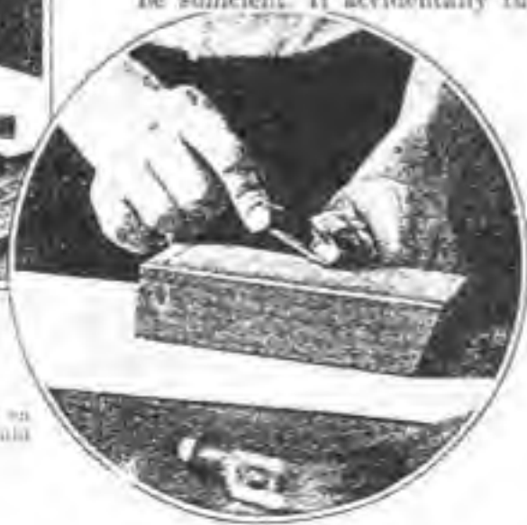
FIG. 4 (above).—How the lips of the bit are sharpened on top by means of an auger-bit file.
