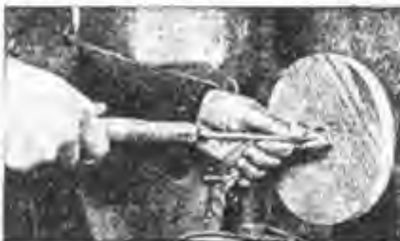
FIG. 47.—Upper view: Using the toe of a skew \frac{1}{4} -in. skew chisel to bore the hole that is to take the tenon of the candlestick upright. Lower view: Marking the diameter of the hole with dividers held on the T-rest and centered by trial.
