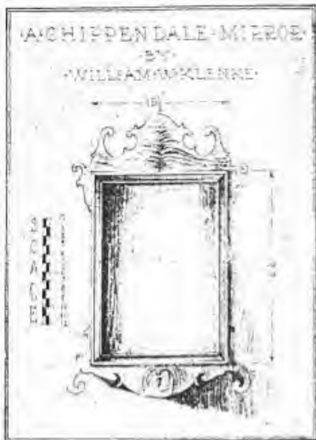
FIG. 20.—Pencil drawing of a Chippendale mirror showing dimensions and style. Details of a section are given in Fig. 21.
