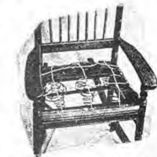
FIG. 14.—The bar and spring method of upholstering a seat. Note how the springs are tied.
