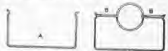
The Shape of the Wire and Manner of Attaching the Rubber Bands to the Ring
