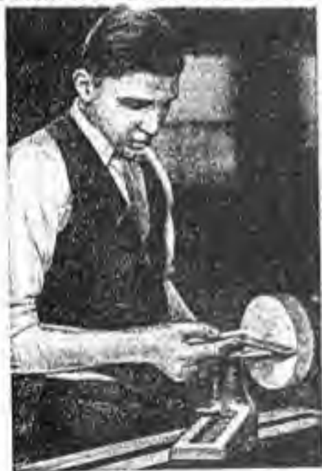
FIG. 46.—After the base has been tried with a round-nose chisel and smoothed with a square-nose tool, it should be tested for flatness.
