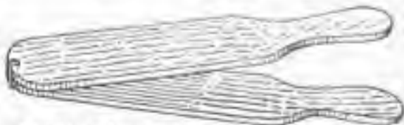
Two Paddles Hinged Together with a Piece of Wire Make a Presser for Lard and Fruits
