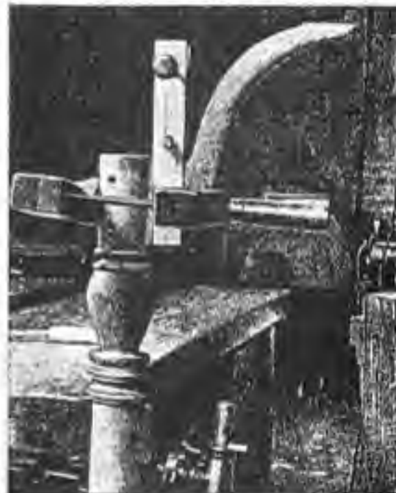
FIG. 34.—One leg at a time is glued to the column and held firmly with three hand screws.
