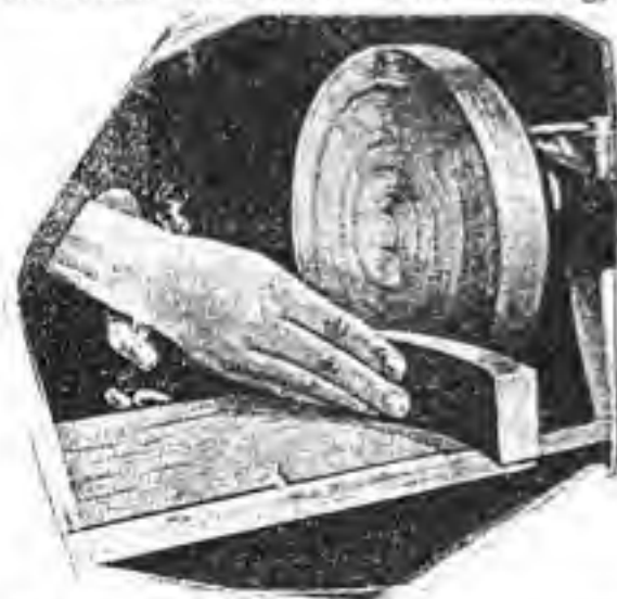
FIG. 70.—How pieces such as the segments of the apron under a circular table top are sanded.
