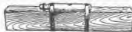
A Bottle Filled with Water and Tied to a Straight Piece of Wood for a Level
