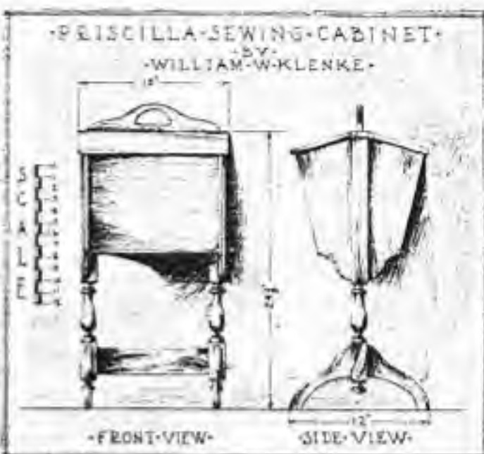
Fig. 10.—The cabinet sketched in pencil. See Fig. 11 for the completely dimensioned working drawings.
