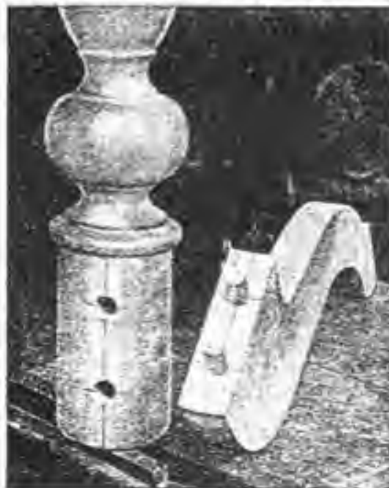
FIG. 32.—One of the legs with dowels inserted, all ready to be glued to the turned column.
