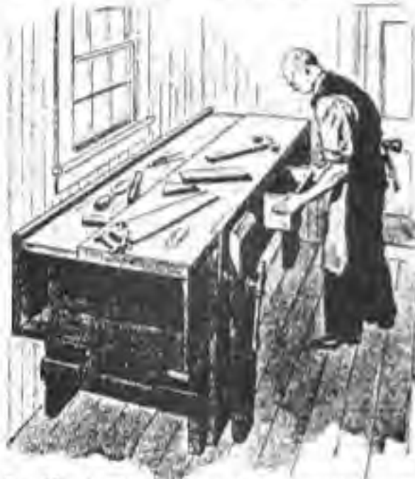
FIG. 17.—A man-size bench of the carpenter's type for the amateur mechanic who does much woodworking and repairing.
