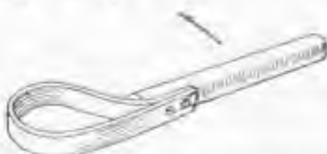
The Loop in the Leather Grips the Cap Tightly When the Handle is Turned as the Arrow Indicates.
