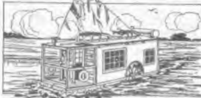
The Hull of the Houseboat is Built on the Scow Type so That It Can Be Run in Shallow Water without Danger
