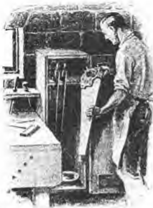
FIG. 41.—The purpose of this cabinet is to protect hand saws from rust and damage.
