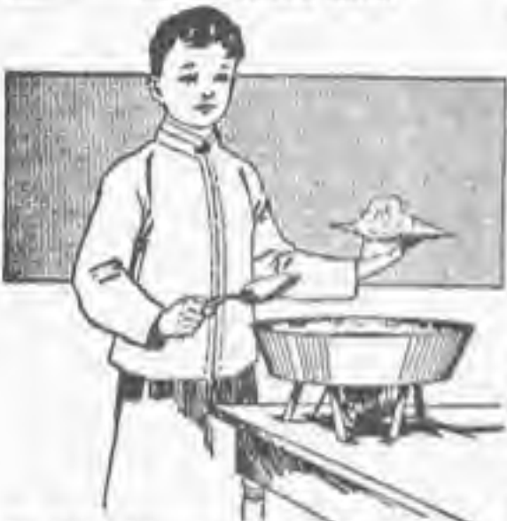
The Disk is Driven by a Small Battery Motor and Melted Sugar is Spun Out into Floss
